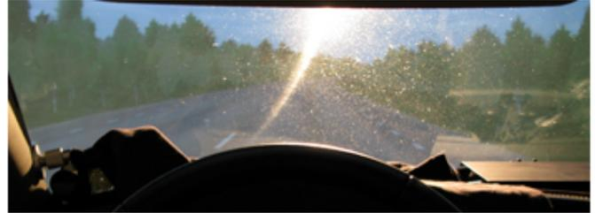
A worn windscreen increases the risk of glare, which may have the result that the driver does not see objects or persons on or near the road in time. This may, in turn, mean that there is less chance of preventing an accident.
